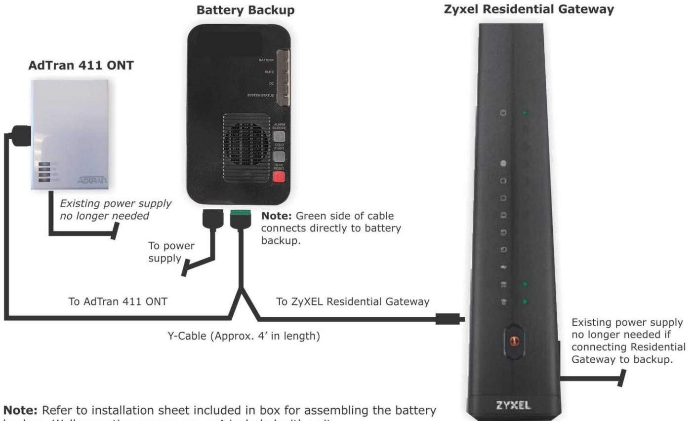
**Note:** Refer to installation sheet included in box for assembling the battery backup. Wall mounting screws are **not** included with unit.
