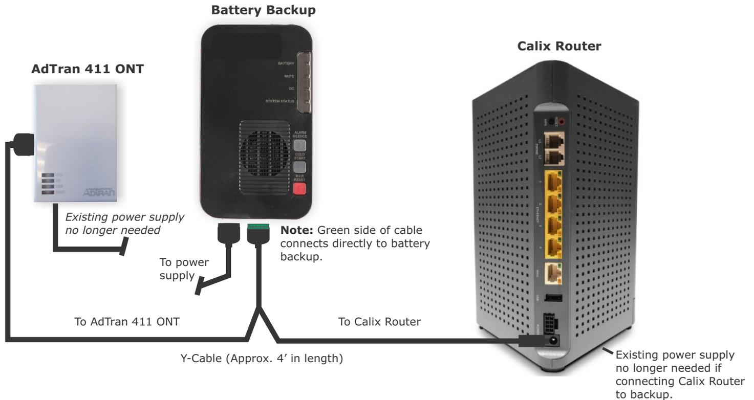
**Note:** Refer to installation sheet included in box for assembling the battery backup. Wall mounting screws are **not** included with unit.
